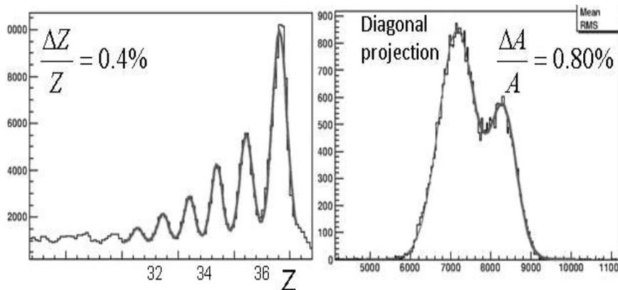
Figure 1. Projectile fragments are identified after the secondary target using the LYCCA array [15]. In the present experiment a stable  $^{84}\text{Kr}$  beam impinges on a primary  $^9\text{Be}$  target to produce different Br isotopes. The Z-resolution (left) of the displayed data [18] is slightly worse than obtained with the FRS detectors. The fragment masses of  $^{83}\text{Br}$  and  $^{84}\text{Br}$  are clearly discriminated.
