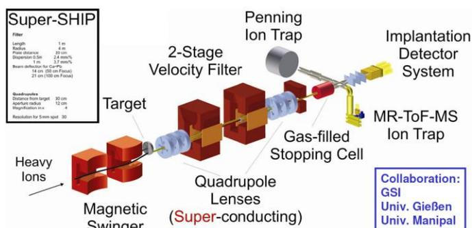
Figure 3. Preliminary sketch of the next-generation, superconducting vacuum separator for transfer and fusion products including advanced instrumentation. It shall be coupled to the planned superconducting cw-linac.
