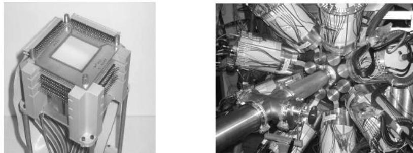
Figure 2. (Left panel) Silicon detector stack of the Beta Counting System. (Right panel) The SeGA array comprising 16 high purity germanium detectors.
