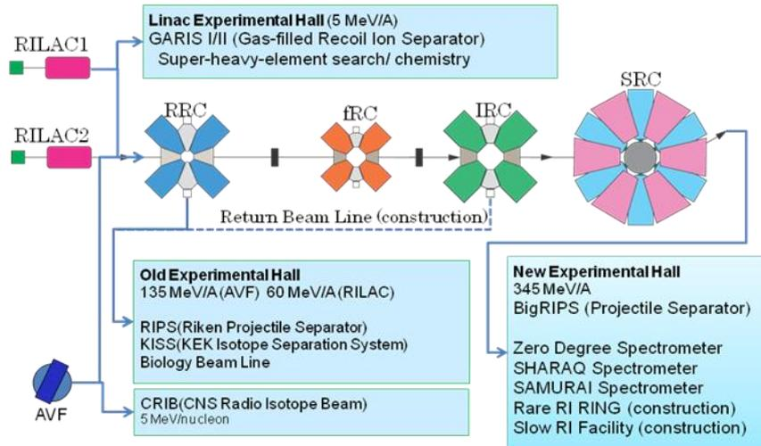
Figure 1: Schematic view of RIKEN Radio Isotope Beam Factory, RIBF. RIKEN Linear Accelerator (RILAC1/2) and AVF Cyclotron are the injectors. RIKEN Ring Cyclotron (RRC), fixed-frequency Ring Cyclotron (fRC), Intermediate Ring Cyclotron (IRC) and Superconducting Ring Cyclotron (SRC) are operated in cascade. Two charge strippers are placed after RRC and fRC.
